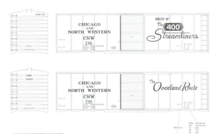
IN 1956 THE PAINT SCHEME WAS CHANGED TO THE LARGE C&NW INITIALS ON BOTH SIDES OF THE CAR.
