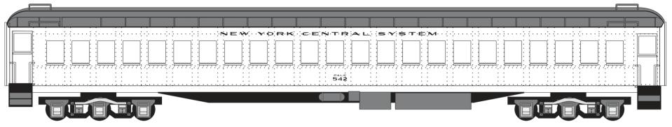
CARS PAINTED BETWEEN 1953 AND 1968 IN 1953 THE PAINT SCHEME WAS CHANGED AGAIN. THE SCHEME WAS CHANGED TO A TWO TONE GRAY SCHEME USED ON THE 20th CENTURY LIMITED AFTER 1946. THE SCHEME IS A DARK GRAY CAR BODY WITH A LIGHT GRAY WINDOW BAND.
