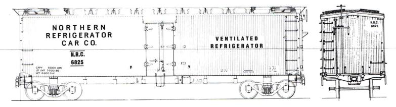
IN 1940 MDT AND NRC CARS HAD YELLOW ORANGE SIDES. ALUMINUM ROOFS AND RUNNING BOARDS. FREIGHT CAR RED ENDS. BLACK UNDERFRAME, TRUCKS AND HARDWARE. AFTER 1945 ROOFS WERE FREIGHT CAR RED.
